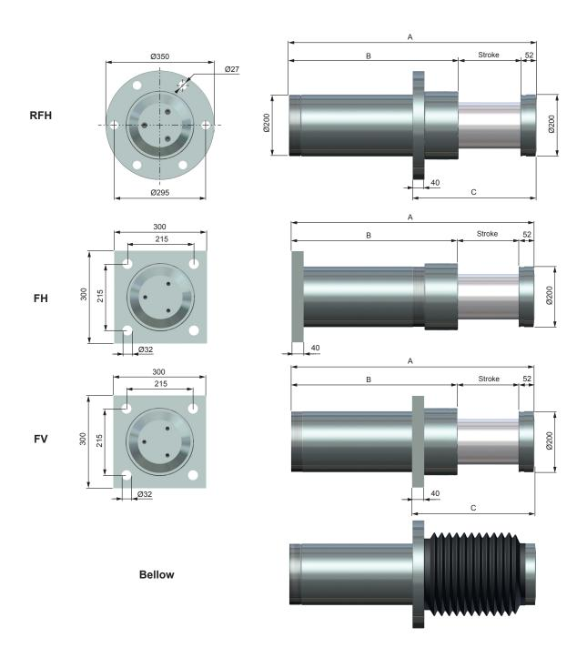
Rear flange recommended only for shock absorbers up to 300 mm stroke!
